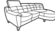
CHAISE END SOFA H100cm (headrest up) H83cm (headrest down) W270cm D179cm SH51cm SW240cm SD57cm AH62cm CSD130cm
